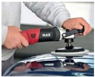
To remove any deep-seated scratches, we would recommend using the polishing lambswool together with FLEX SpecialPolish.
