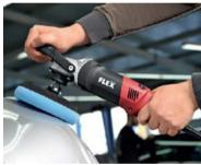
2. Scratches can be removed using the blue polishing sponge and FLEX SpecialPolish.
