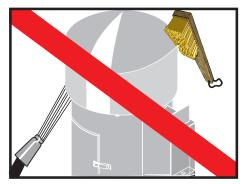
Inspect vacuum exterior. Clean equipment invites usage. Rinse with plain (preferably softened) water as necessary. (Be careful not to spray water upward under the dometo-tank vent areas). DO NOT USE STEEL WOOL OR OTHER FEFFOUS BRUSHES TO CLEAN STAINLESS STEEL SURFACES.
