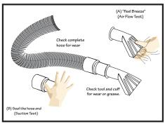
Check hose for signs of wear, replace if excessive. Test vacuum suction and airflow. Suction test: place hand tighly over cuff - feel for "pull".
