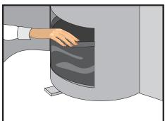
Remove dirt and debris from vacuum. HINT: Consider ordering a debris catcher (p/n 100700) from your distributor to simplify this process.
