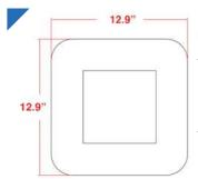
The SCRT includes an LED panel and a high rise driver lid, both of which fit in a previously installed Scottsdale<sup>†</sup> fixture. This product is sized as a retrofit kit and is not for new installation.
