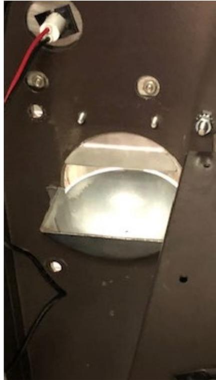
REMOVE THE BOTTOM PLATE AND FLIP DOOR ASSEMBLY
