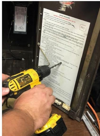
■ USING A LETTER "F" (.257") DRILL BIT, DRILL THE TWO HOLES IN THE DOOR AS REQUIRED
