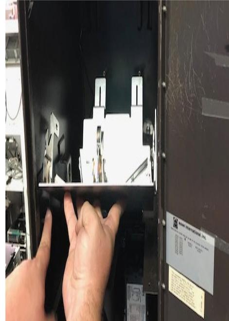
■ TILT THE ASSEMBLY AT AN ANGLE AND INSERT INTO THE MACHINE SO THAT THE SIDE TABS ARE AIMED AT THE SIDE BRACKETS OF THE CABINET AND CAN REST IN THOSE EXISTING BRACKTS
