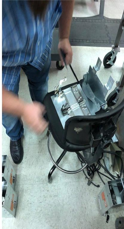
■ REMOVE THE TWO HOPPERS FROM THE ASSEMBLY TO MAKE IT LIGHTER AND EASIER TO INSTALL
