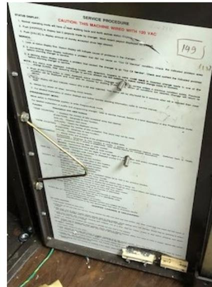
■ INSTALL QTY.2 1/4-20X3/4 HEX BOLTS INTO THE HOLES WITH THE THREADS ON THE INSIDE OF THE DOOR
