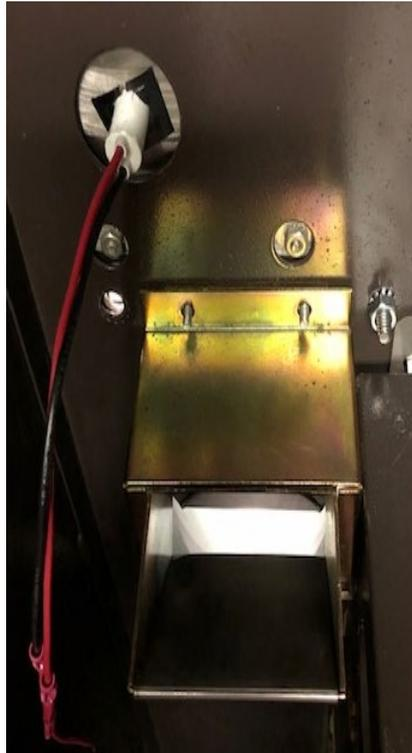
■ INSTALL THE TOP RETAINING PLATE AND SECURE THE ASSEMBLY WITH THE NUTS THAT WERE REMOVED EARLIER
