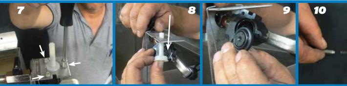
With 1/4" Nut Driver remove the 3 screws that hold Valve Body to Bracket.
