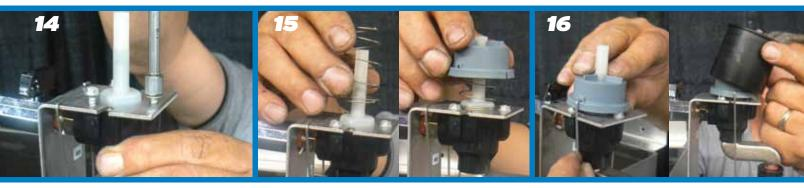
Re-tighten the 3 screws that hold Bracket and Valve Body together.
