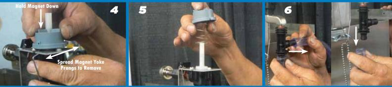
Hold down on Magnet and remove Magnet Yoke.
