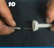
Inspect, clean and/or replace Plunger and Spring Assembly.
