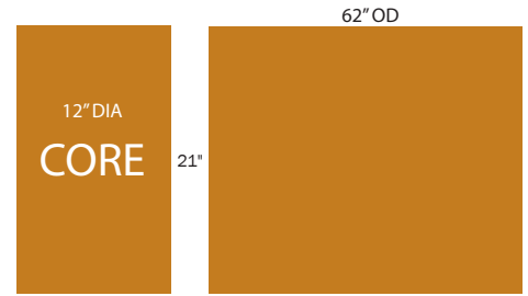
HORIZONTAL WINDOW WASHER 12 X 21 X 62 STRAIGHT CUT FIVE STAR CAR WASH FOR HANNA
