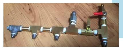
Compressed air, with a small amount of water introduced by the ball valve, is key to generating the nucleation (see below for explanation) particles that mix with the pressure washer spray from the 4002 tips. The check valve is to prevent water from going back into the compressor and potentially damaging it. The process won't work without the high-pressure air or water."
